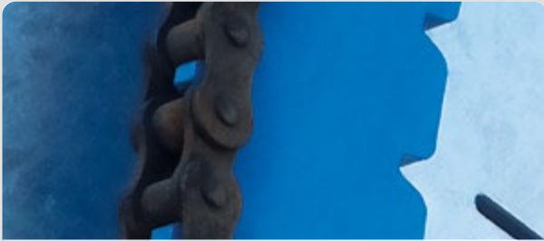
Uncoated chain gets heavily corroded due to exposure to various environmental influences (e.g. rain, road salt, salty air in harbours)
