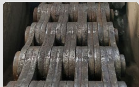
FB log-gripper chain after 12 months of use
