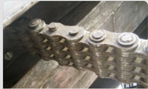
Massive damage to the pins and washers after only 3 months
