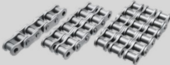
Roller chains with chamfered plates ISO 606 (DIN 8187, DIN 8188) and FB-factory-standards – simplex, duplex, triplex
